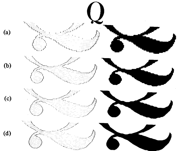
Fig. 6. Telescoping template enlargement, s_x = s_y = 5.5 . (a) Result of 0th-order scaling. (b) Result of first-order scaling. (c) Result of second-order scaling. (d) Result of third-order scaling.
