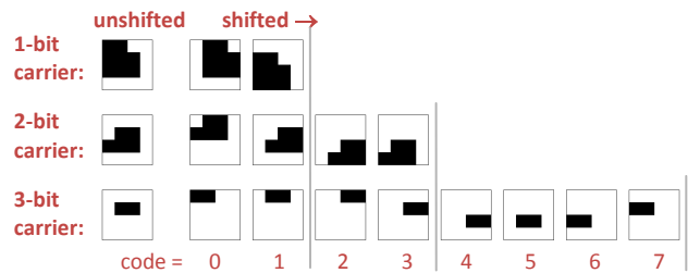
Figure 4. Shift positions for 1-, 2-, and 3-bit codes as defined by the Carrier Shift Rule.
