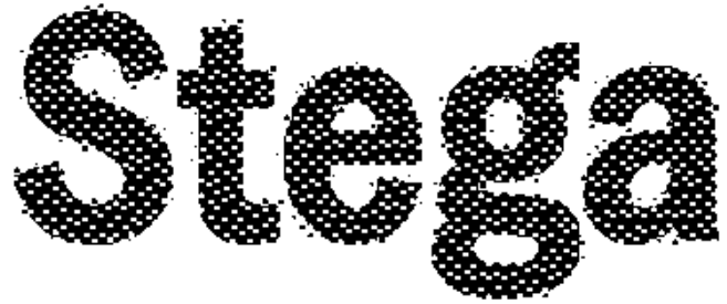
Figure 5. Portion of a Stegatone of the logo from Figure 2 revealing noisy edges.
