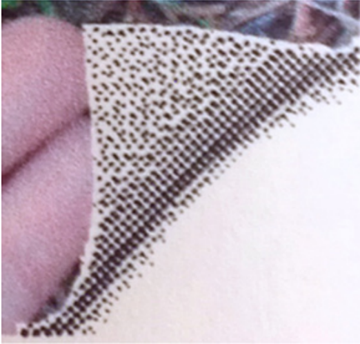
Figure 2. An enlarged view of a captured data-bearing “flip-up” graphic; the capture and subsequent reading process is used to extract information from minute perturbations.
