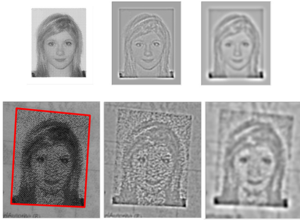
Figure 10. Successive difference-of-Gaussian representations of reference halftone (top), and captured stegatone (bottom).
