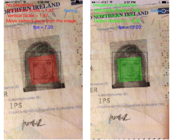
Figure 11. Mobile UI of fast stegatone detector. Screen captures from an iPhone 5S.
