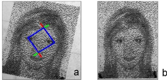
Figure 6. (a) Reconstructed East and West cardinal points using approximate North and South cardinal points plus calculated vanishing points; (b) Dwarped image using homography calculated from the 4 transformed cardinal points.
