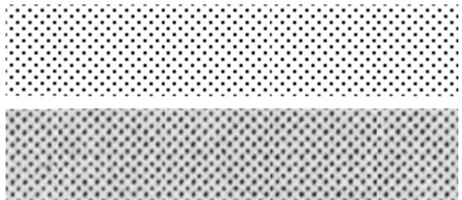
Figure 1. Digital 45 degree 12.5% halftone screen (top) and a similar scanned print from a HP LaserJet 1200 (bottom).
