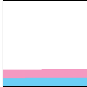
Fig. 3: A halftoned patch of a constant NPac of 80% blank media, 10% of one drop of magenta and 10% of one drop of cyan over an area of 128 x 128 pixels.
